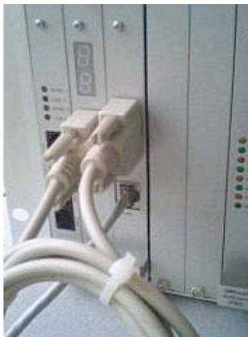
Figure 21: Connection between IPG and CPU board (non-hotplug backplane)
